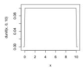
A plot of the probability density function for the uniform distribution looks like a plateau. Note that the PDF is normalized, so that the area under the curve is unity. Also note that the plot that R produces is an approximation; the edges of the plateau should be perfectly vertical.
