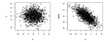
It seems that there is a strong relationship at work here, but it is all a fallacy. The x and y values are completely independent. The regression was  $\Delta$  against x, and  $\Delta$  is not a separate measurement from x. This phenomenon is often referred to as 'regression to the mean'.
