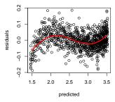
Here we see a clear pattern in the residuals. This is an indication that the model is not explaining the data well. While we could probably use the pattern detected in the residuals
