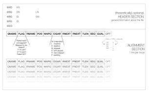
Each line of the optional header section starts with Q. and includes information such as chromosomes names (SN) and their lengths (LN). The vast majority of lines within a SAM file are compact representations of the read alignments where each read is described by the 11 mandatory entries and a variable number of optional fields [Li et al., 2009].
